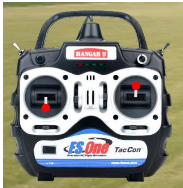
Figure 4. Right control stick pushed forward—plane pitches down.
