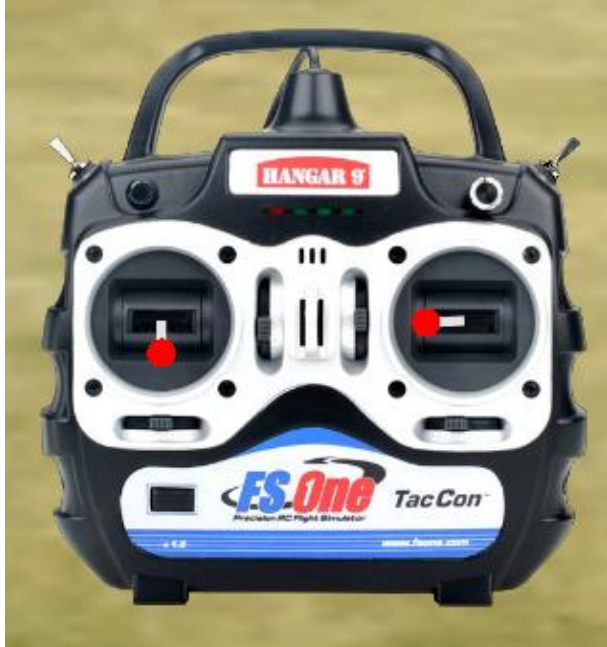
Figure 5. Right control stick moved left. Plane banks left.
