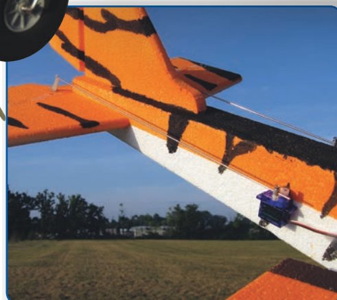
Tom Sullivan mounted the elevator and rudder servos on the fuselage, just behind the wing.
