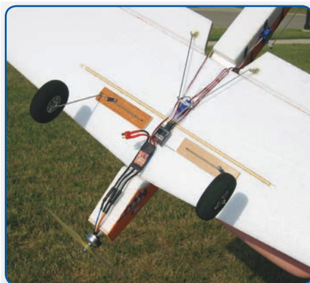
Locating the receiver, aileron servo and ESC on the underside keeps the upright appearance cleaner.
