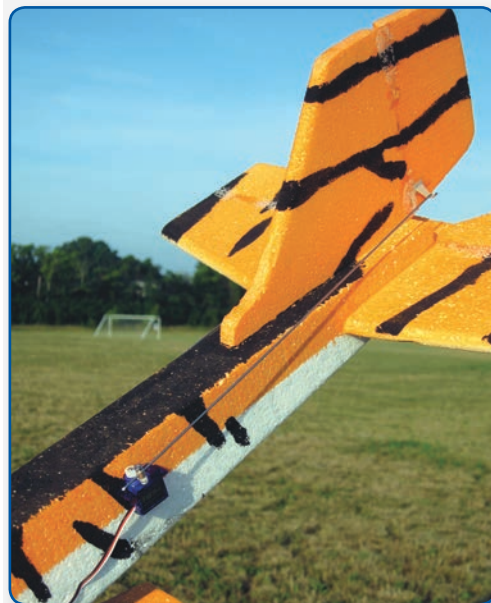
The rear-mounted tail servos help balance the model on the CG. Shorter pushrod runs help to reduce flex.
